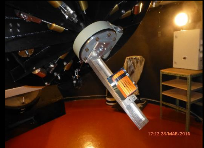
The Raptor "Ninox 640" InGaAs camera at the F/12.5 Cassegrain focus of the Omicron@C2PU telescope
