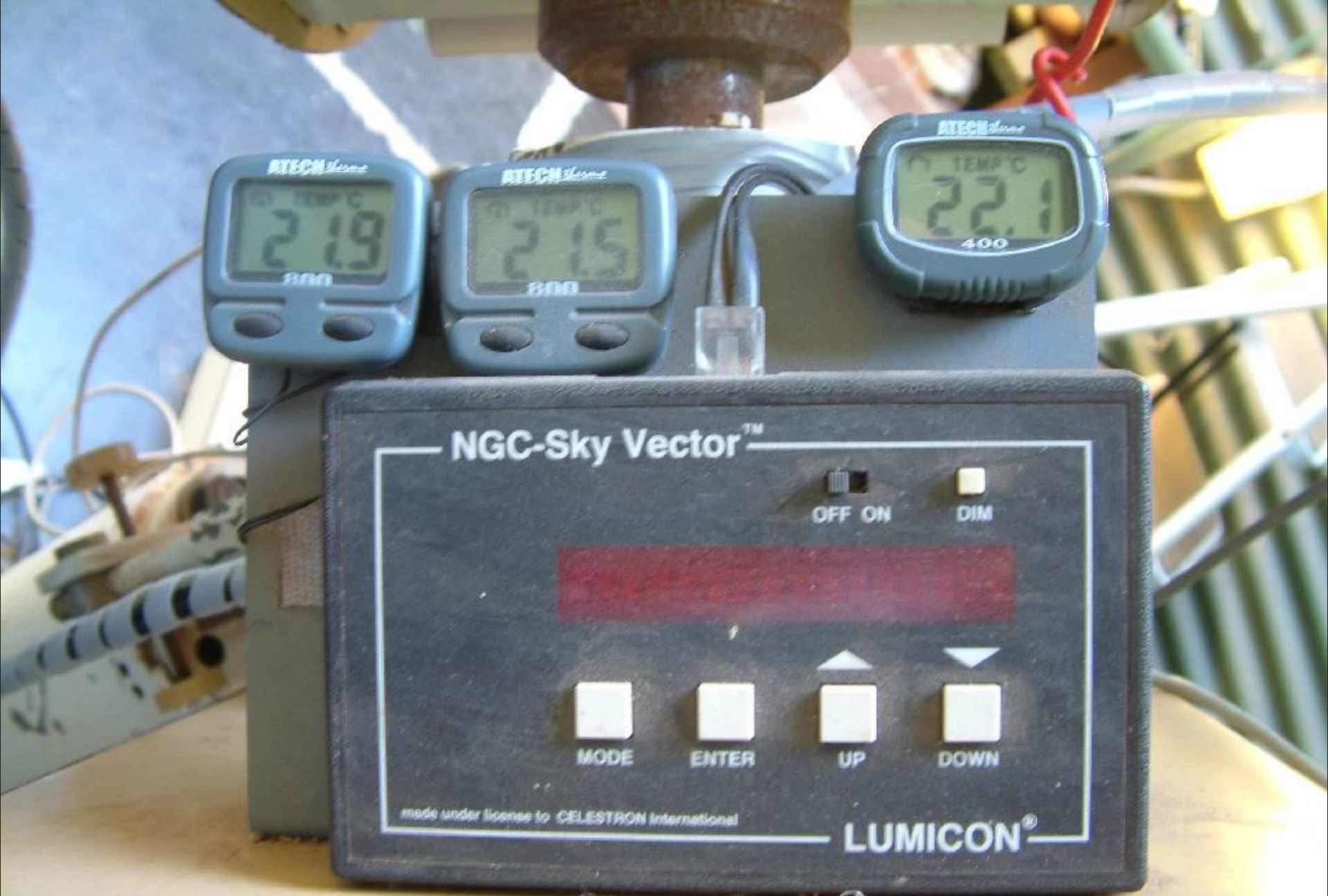
Digital thermometers, from the left, the temp of the back of the primary mirror, the temp of the side of the primary mirror, the ambient temp in the observatory.
